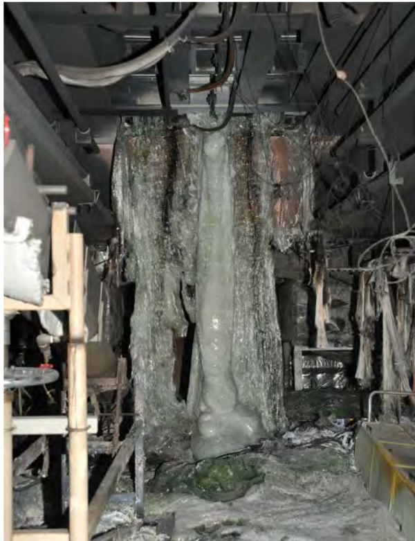
Damage from molten glass tank overturning in Japan
