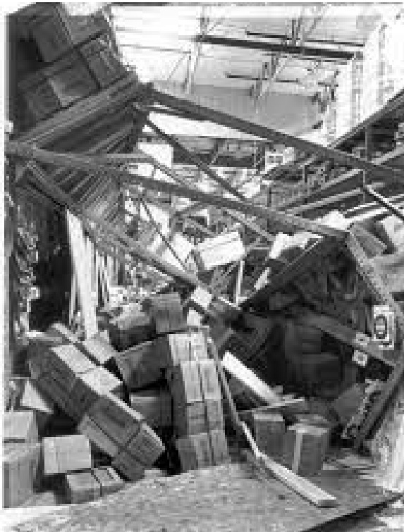
Storage Racks in 1994 Northridge Earthquake
