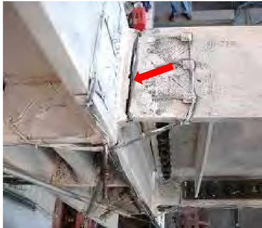
Pre-Northridge Moment Frame Connection Failure
