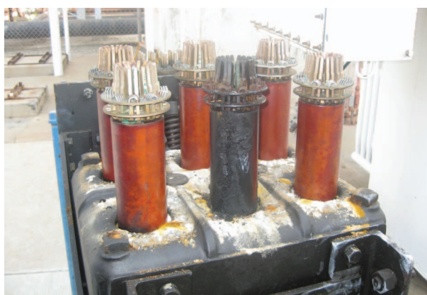
FIGURE 1. A distribution breaker with burned-out pole insulation. (Photo courtesy of the Tesoro Corporation.)
